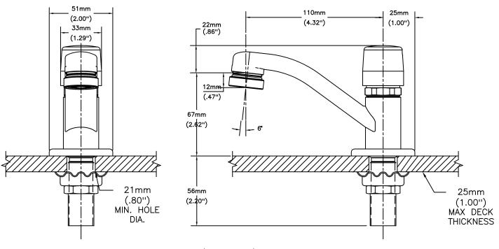
INLET FOR 3/8" OR 1/2" FLEXIBLE RISER OR 1/2-14 NPSM COUPLING NUT (NOT SUPPLIED)
